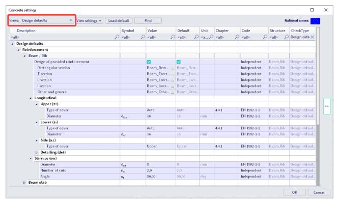
Several default templates for longitudinal reinforcement and stirrups are available for the different section types (provided reinforcement). These can be changed, or new ones can be made.
