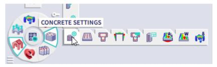
Templates of longitudinal reinforcement and stirrups for different shapes of beam are available. The concrete cover can be set for upper, lower, and side faces.
