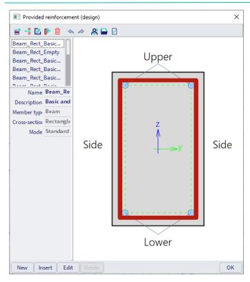
This template exists of basic, additional and shear reinforcement. The purpose is to compare these templates with the required reinforcement, to model the user reinforcement that is introduced later or to convert it automatically to user reinforcement.
