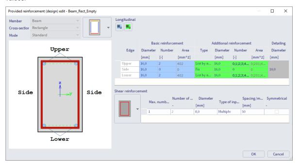
This means that in the provided reinforcement we always have the basic reinforcement of 2 bars – on the upper and lower edge – of diameter 16mm. This can be increased with the values of the additional reinforcement. However, this will only be increased if the provided reinforcement is less than the required reinforcement. This comparison will be done for each section of the beam.
